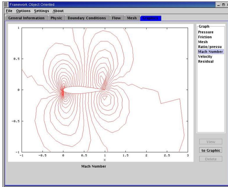
**Fig. 5. NACA 0012 Airfoil Mach Number Lines**
